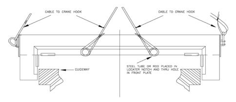
IT IS VERY IMPORTANT TO ENSURE THAT THE SIDE GUIDE SHOES DO NOT COME TO REST ON THE GUIDEWAYS WHEN MOUNTING THE STEEL COVER
